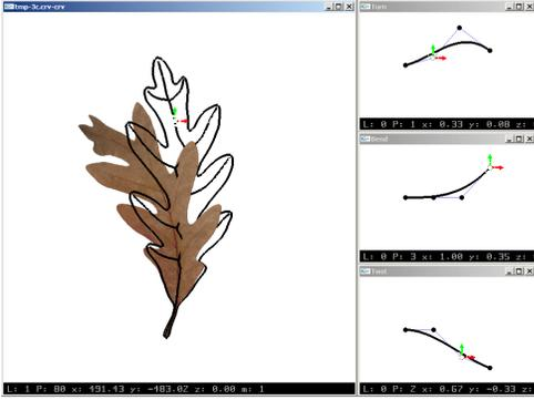
**Figure 6. A screen shot of the modeling environment. The leaf model can be deformed in 3D space using graphically defined functions that control additional turning, bending, and twisting of the skeleton.**
