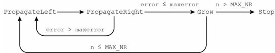
Figure 2. The sequence of phases in the simulation of a growing and bending branch. Similar graphs are useful when defining the sequence of phases in other L+C models as well
